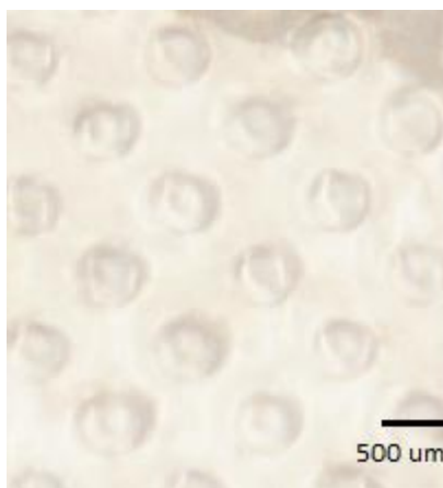
Figure 3.3: The top view photograph of PDMS sheet with holes created by the mold shown in Fig. 3.2.
